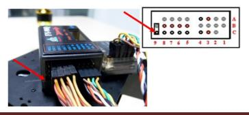
Orientate the FY90Q so that the arrow points **between** Motor No. 1 and No 4.
