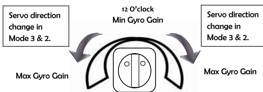
2. **Gyro Gain:** The further away from Centre (12 O' clock) the higher the Gyro gain (sensitivity). Too low gain result is poor auto stabilization, too high gain will cause oscillations of the aircraft. You need to adjust the gain setting based on the requirement of your aircraft.
